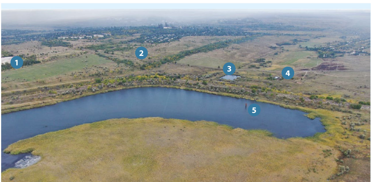
Figure 25. Sludge SF No. 2 and other facilities: ❶ Inkor sludge SF No. 1, ❷ vehicle road, ❸ earthen reservoir, ❹ pump station, ❺ water intake tower. Photo: OSCE, 2019
